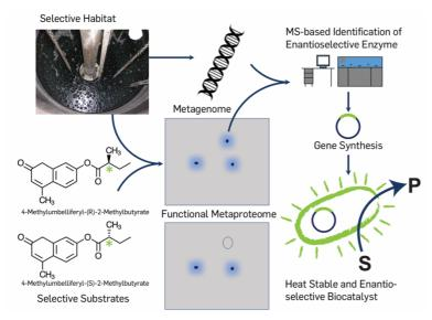
**Exemplary functional metaproteomics pipeline**: Proteins and DNA from a promising habitat (e.g. a hot spring) will be isolated. Proteins will be separated on 2 D gels and screened for activity using tailor-made fluorogenic substrates. Enantiospecific biocatalysts will then be excised from the gel and identified by mass spectrometry. Through synthetic biology the biocatalyst will be obtained in quantity for characterization.
